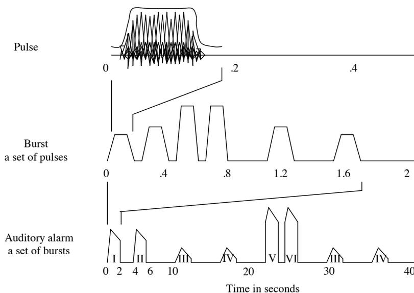
Figure 19.1: Design of alarms according to Patterson. The alarm consists of bursts that consist themselves in sets of pulses.
