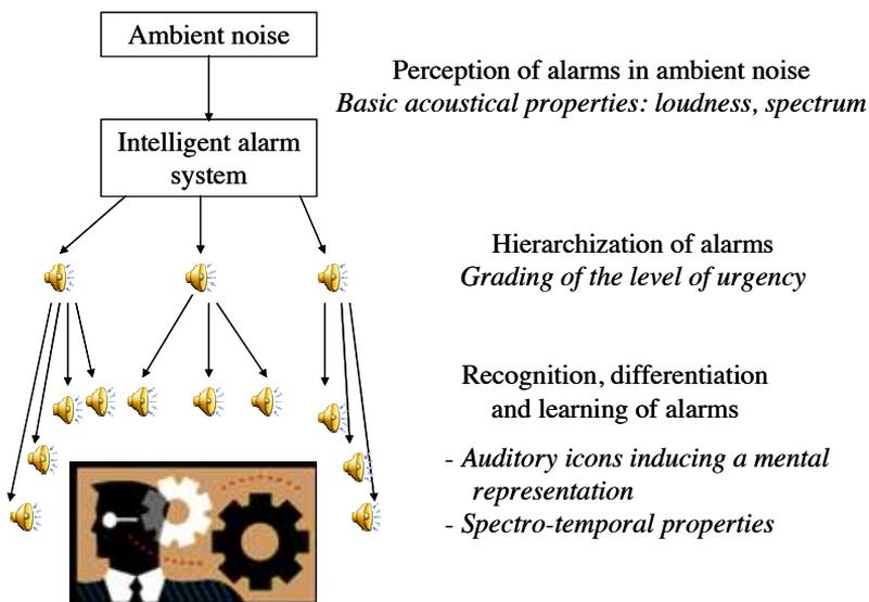
Figure 19.2: General scheme of an intelligent alarm system.
